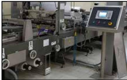
Side-Mounted Operator Control Panel
